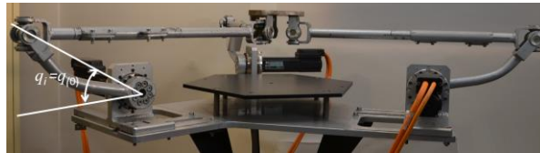
Fig. 1. View of the 3RUU manipulator in the analyzed singular configuration
